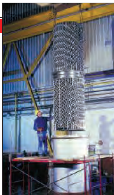
FIGURE 3. The Sulzer Mixer Reactor (SMR) is a tube-bundle heat exchanger that allows high-effective cooling or heating of viscous media. The SMR is a suitable choice to combine effective mixing with controlled heat transfer
