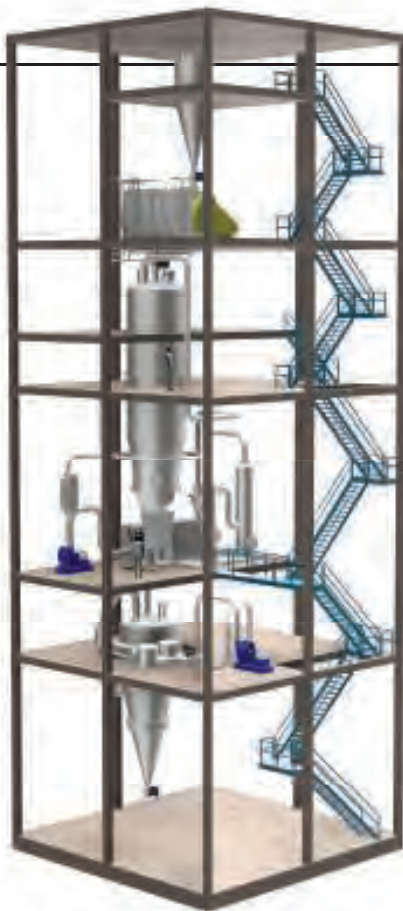
FIGURE 4. The BePET process is said to be stable, efficient and reliable with no high-maintenance vacuum or extrusion decontamination required. The design promotes uniform plug flow and minimizes the potential for short-circuiting
