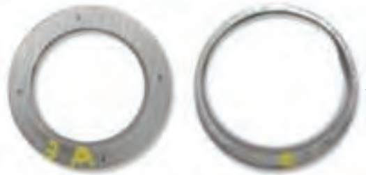
FIGURE 2. Tubewall thinning is caused by single-phase FAC
