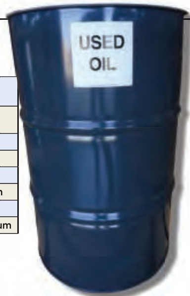
FIGURE 2. Used oil should be stored in clearly labeled drums
